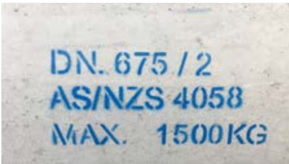
Example of marked pipe. Note: the date and precaster name has been removed.
