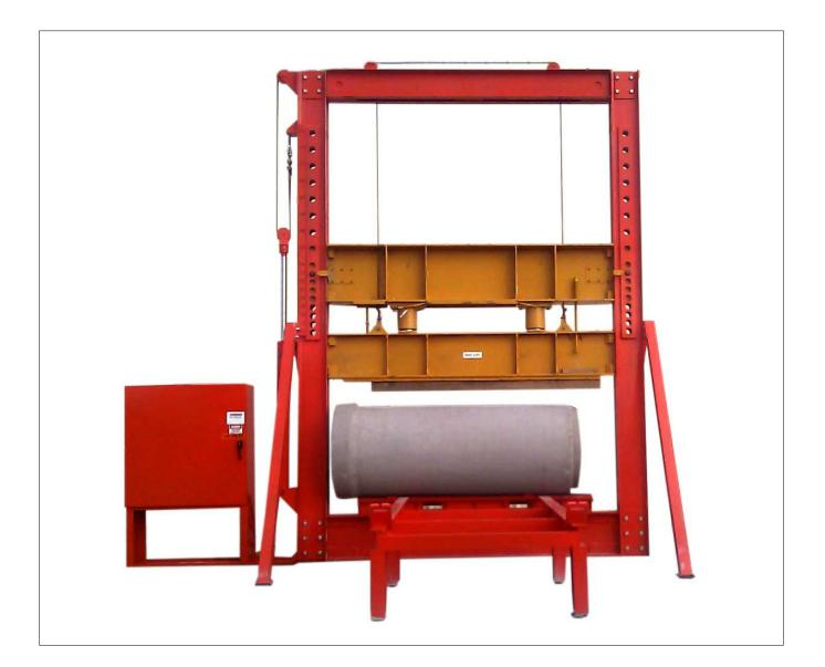
EKOPipe production batches have been tested for both proof and ultimate loads in accordance with AS4058, and all EKOPipes exceed the load requirements listed in AS4058.
