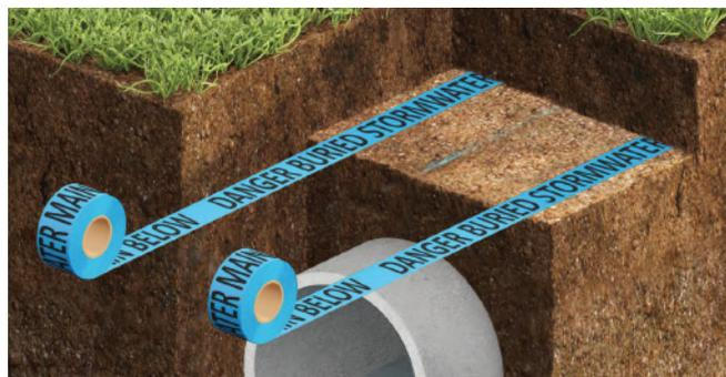
Figure 3 - Warning tape installed above select fill - preferably two runs either side of the trench.
