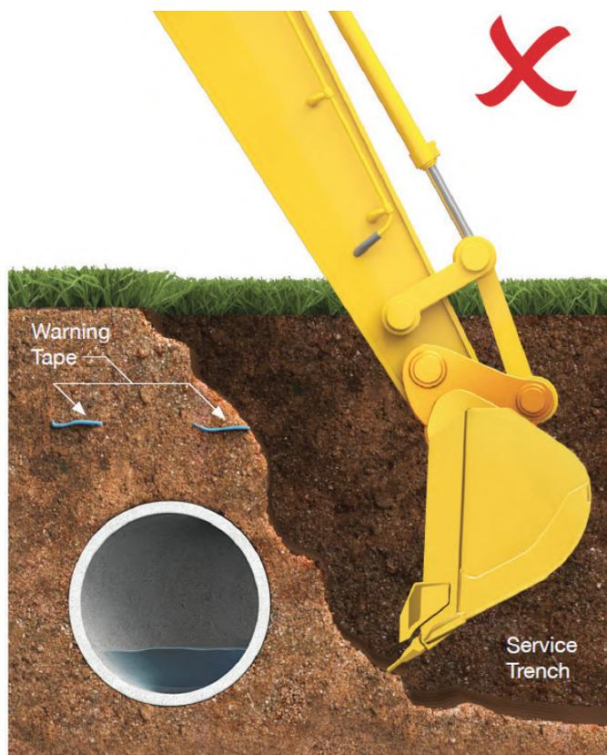
Figure 6 - Typical excavation direction - can cause damage before pipe is uncovered.
