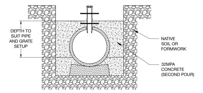
Figure 15 – Second Concrete Pour
