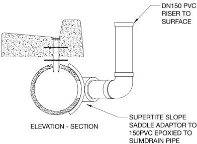
Figure 4 - Flush point cross section
