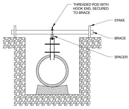
Figure 11 – SlimDrain bracing detail
