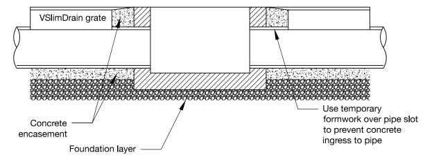
Figure 18 – Connection to Pits
