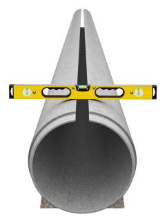
Figure 8 – Pipe slot level
