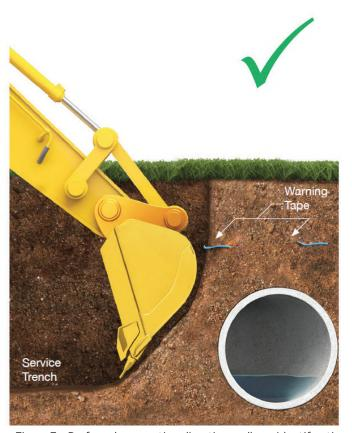
Figure 7 - Preferred excavation direction - allows identification of pipe before damage occurs.
