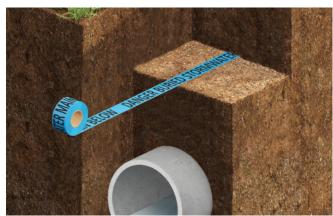
Figure 2 - Warning tape installed halfway between surface level and top of pipe
