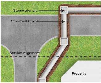
Figure 1 - Example of Service Alignment Crossover
