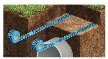
Figure 3 - Warning tape installed above select fill - preferably two runs either side of the trench.
