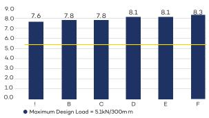
This test far exceeds the requirements of typical pipe service requirements, as the maximum design load for a DN375 Class 2 pipe is 5.1kN/300mm. This equates to a load of 520kg for a 300mm pipe length.
