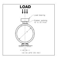
Samples of saturated pipe specimens were placed under constant load in a load testing rig, with loads ranging from 775kg up to 850kg (actual weights 775, 800, 800, 825, 825, 850kg). These load testing rigs and pipes are submerged for the duration of the testing.
